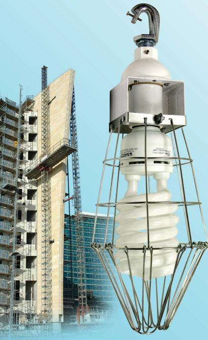
The Temporary Work Light fixture with a mogul base is used to protect a 105w Compact Fluorescent Lamp. Available for 277 volt electrical systems, the fixture comes with a hook and a 5´ blunt-cut cord. The lamp is self-ballasted, eliminating the need for an additional ballast.
