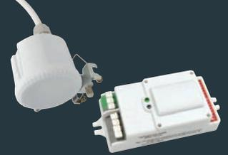
Microwave Technology sensors offer advantages over Infrared Technology sensors for outdoor and warehouse applications because they are NOT affected by ambient temperatures above 90°F (32°C). Infrared sensors read temperature signatures as people cross activation zones near the sensor. When the ambient temperature is close to human body temperature, the sensor does not see motion.
